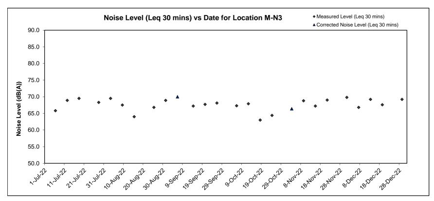
Remark: 1. The Contract no. HY/2018/08 Central Kowloon Route – Central Tunnel commenced on 19 September 2019. 2. Corrected Noise Level = 10\* log(10^(Measured Noise Level/10) – 10^(Baseline Noise Level/10))
